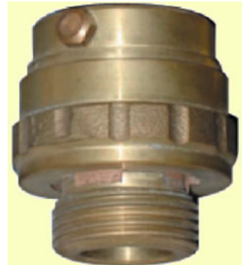
Hose bib vacuum breakers insure that non-potable water or contaminants are not siphoned into potable water supply and are available at most hardware stores.
